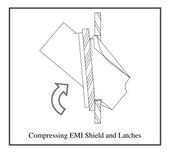
**4.** While applying downward pressure to the adapter, continue rotating the adapter toward the faceplate, until the latch(es) clear the panel opening and catch on the upper edge.
