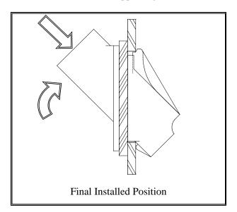
**5.** Apply upward pressure on the front face of the adapter, sliding it up. This insures full overlap of the latch(es) on the faceplate.
