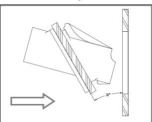
**2.** While placing the adapter through the faceplate opening, hook the adapter on the bottom of the faceplate opening.
